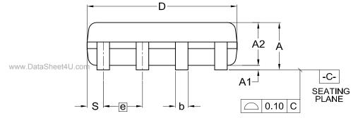
Dimensions (inch dimensions are derived from the original mm dimensions)
