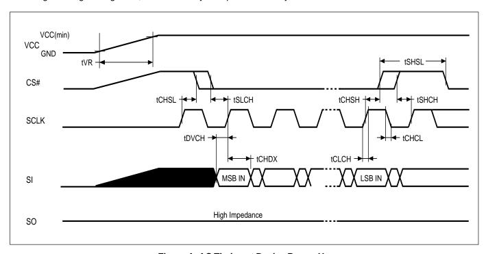
Figure A. AC Timing at Device Power-Up
