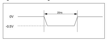
Figure 4. Maximum Positive Overshoot Waveform
