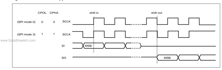
Figure 2. SPI Modes Supported
